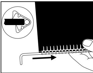
2. With bar side up, center lacing on belt holding belt against gauge pin.
