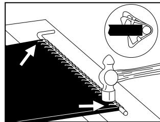
3. Using a soft wood surface for support, hammer end teeth halfway into top of belt.
