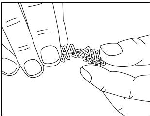
I. For belts narrower than 12" (300 mm) break or cut the lacing to size.
