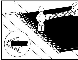
4. Turn belt over and hammer lacing halfway into bottom of belt.
