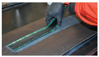
7. Apply repair strip to damaged area making sure to apply the center first.
