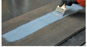
6. Apply "tack" coat to prepped surface and to the back of the repair strip.
