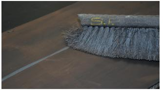
1. Using a Foxtail Dust Brush, remove debris and loose material from damaged and surrounding area to prepare area for buffing.
