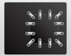
Larger size holes can be effectively repaired by applying standard Flexco<sup>®</sup> solid plate fasteners and a patch of belting as shown.
