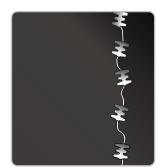
For quick temporary repairs, hammer-applied Turtle (TM) No.16 fasteners are recommended every four to six inches (101 to 152 mm) along the rip.
