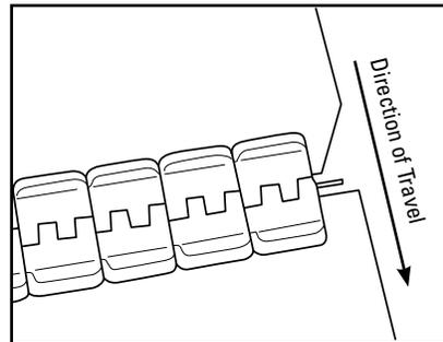
11. Mesh the two belt ends together and insert the hinge pin. Notch the trailing belt end, and, using pliers, bend the end of the pin to prevent migration.
