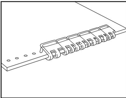
4. Install the fasteners across the belt by opening each plate enough to slide it over the belt. Insert the rivets from the top placing the smooth side of the fasteners on the top side of the belt. Squeeze each plate to make certain that it is inserted fully.
