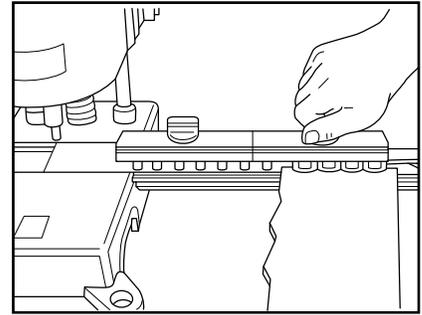
9. Remove the gauge pin, loosen the clamp screws, and remove the belt from the comb assembly. Repeat the procedure on the second belt end.
