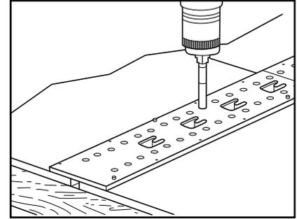
3. Install the appropriate belt punch in the chuck of a 3/8" electric drill. Spray Alligator Plastic Rivet Lube in the holes of the templet and drill the holes in the belt. Do not punch holes up to the edge of the belt. Leave 1/4" of belt open for notching.
