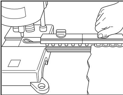
**10. Installing fasteners on a wide belt:**
