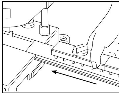
5. Insert the proper comb assembly into the MDT-1 installation tool and make sure that the proper curling bit is installed in the MDT-1. Connect the installation tool to a 110 volt outlet.
