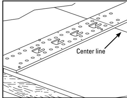
2. Place templet over belt end, aligning centerlines and, make sure belt end is tight against templet lugs. Slide second belt end under templet, against lugs. Align centerlines. Nail or clamp the templet in place.
